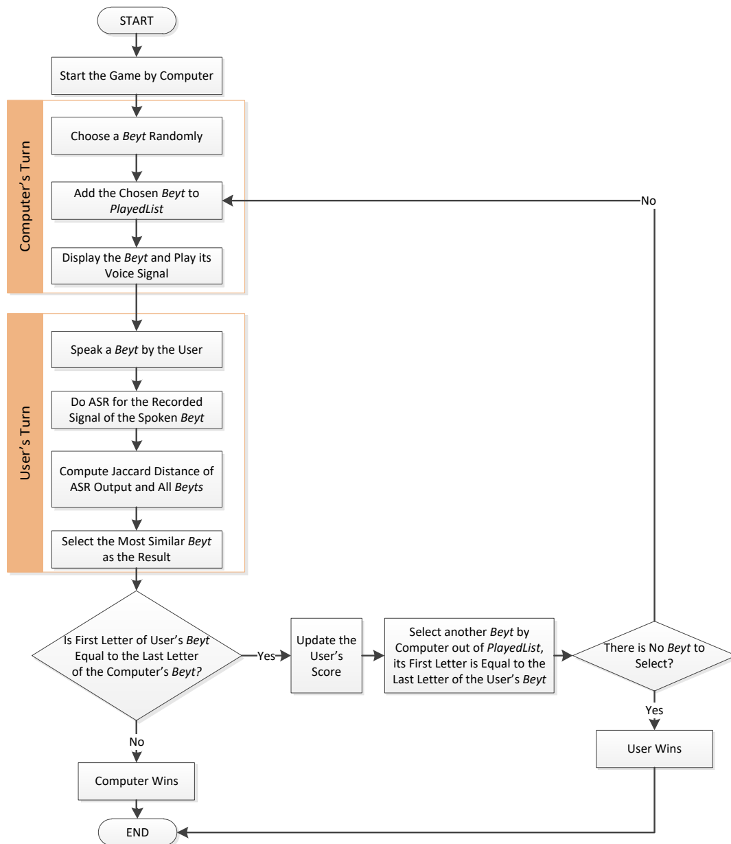
Figure1: The flowchart of the proposed Mosh'a'ere system (Chakame)
